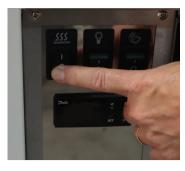
Step 1 **IMPORTANT:** turn off the MCC by pressing the O on the 3 switches. Pull the plug.
