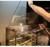
Step 4 Lift and hold the top glass pane while removing the transparent air guide pane for cleaning.
