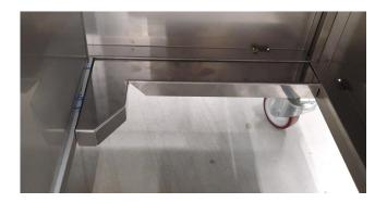
Support mounted in correct position in the under-frame.
