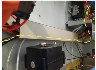
Lead the cable from the swivel trough the cable tray to the connection terminals.
