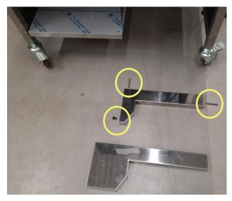
Mount the Caddy support in the underframe with 2x M8x55 + Toothed spring washers and 1x M8x20 bold.
