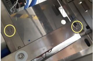
Fix the plate from below with 1x M8x55 + Toothed spring washer and 1x M5x20 bold.
