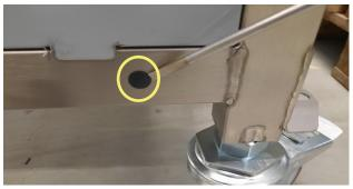
Fixation holes might be covered with plastic caps. Remove the caps with a screwdriver.
