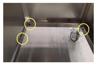
Use the yellow marked fixation points/holes in the under-frame.
