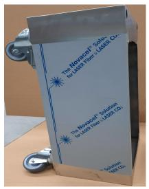
Take the Grease Caddy housing and put it on the backside. (Use some cardboard to prevent damage)
