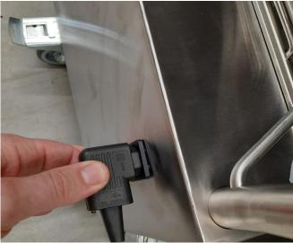
Connect the cable to the Grease Caddy 24V-socket.
