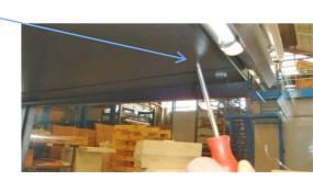
4) secure the temperature indicator with 2 screws. Max. length of screws is 15mm
