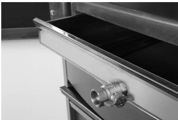
Drain valve open. (Handle horizontally)
