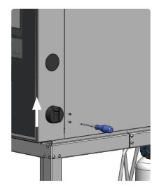
5. Fasten the holder to the right-hand side of the oven using two screws and an Allen key.
