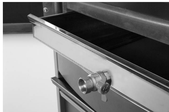
Drain valve closed. (Handle vertically)
