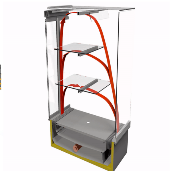
Hot air flow Full Serve
