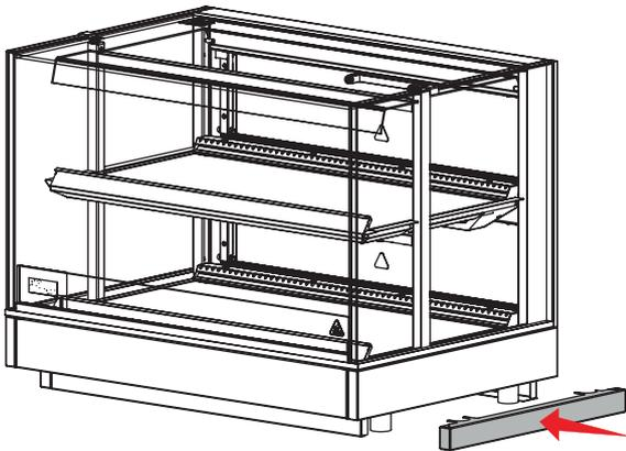
3. Close everything up by placing the second side plinth around the legs, snapping into the back and front plinth.
