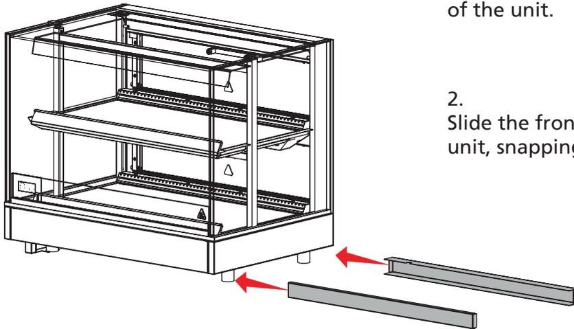
2. Slide the front and back plinths underneath the unit, snapping them into place.
