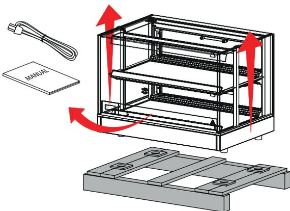
4. Take the manual, power cord and the unit out and lift the unit from the pallet onto the counter.
